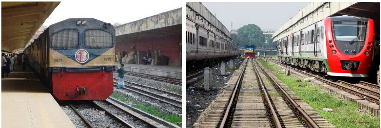
(Bangladeshi model of upgrading railway infrastructure by introducing two-in-one gauge system)
